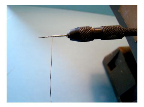
Once the entire bit has wire coiled around it, place your thumb and fore finger on the wire at the base of the coils, at the bit and the pin vise, and slowly pull the coils off the bit. Trim any excess wire that was not used to make the coil and you now have an oxygen hose ready for installation and painting.
